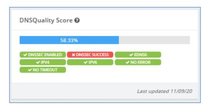
DNSQuality checks are grouped into badges, which represent a group of tests. The badge will be green for successful tests and red for failed tests.
